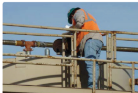
A worker collecting a sample from the open hatch of a production tank. Image: J.D. Danni, OSHA.
